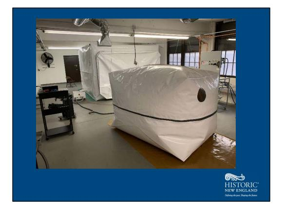
Along with the large or "Mama" bubble, Bill also provided us with a smaller "Baby" bubble which can hold about 175 cubic feet of material and does not have a framework so it can collapse fully. This is an advantage for treating smaller boxed or created material. We can vacuum the membrane tightly around the material and then only need treat the volume of what's inside rather than the commitment of full volume in Mama bubble.
