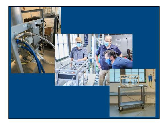
Pat Kelley and his colleague James Feston also came to personally install the introduction system which included a remote switch allowing us to turn on or off the nitrogen flow from anywhere with a computer or smart phone and a custom-made humidification system to ensure the very dry nitrogen does not shock materials inside upon introduction.
