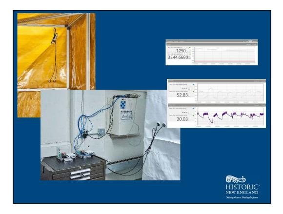
Pat and James also installed the monitoring system for the Mama and baby bubbles. The sensors and software is provided byt the company Rotronic. The monitoring system will allow for Temperature Relative Humidity and  $O_2$  to be monitored in person or remotely using cloud technology.
