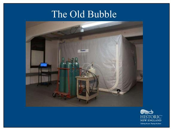
For nearly 30 years, Historic New England has used a thousand cubic foot CO2 based treatment facility effectively for internal use and for outside clients. In 2019 we began seeing signs of wear and inefficiencies in the system and began researching and update and possible replacement to the system.
