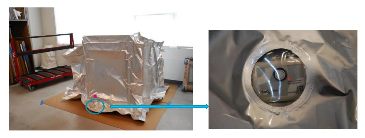
The oxygen monitor will flash red until oxygen drops below the required level (may take up to 72 hours)
