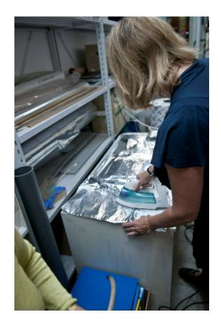
Withdraw the vacuum nozzle and seal the bag
