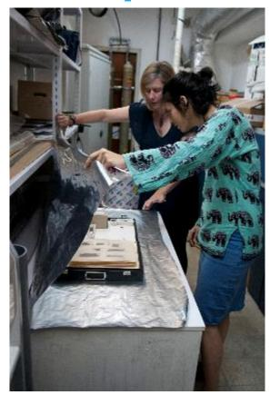
The material to be treated is laid out on the film. In this example the artifacts were treated in their storage box to provide protection during treatment
