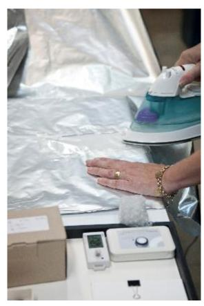
A small window can be created using Escal to allow for reading the oxygen and temp/RH monitors
