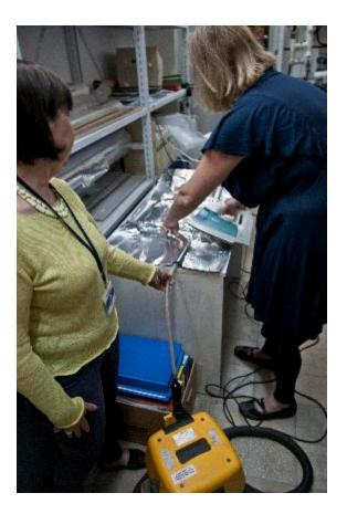
Use the vacuum to draw out oxygen before fully sealing the bag
