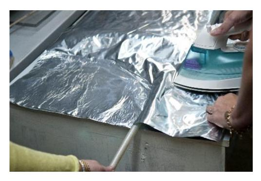
Start sealing the film using an iron, tacking tool or crimper. Leave space for the vacuum hose or nozzle.
