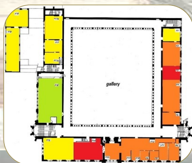
Figure 1– Floor plan of OUMNH first floor, with risk zones
