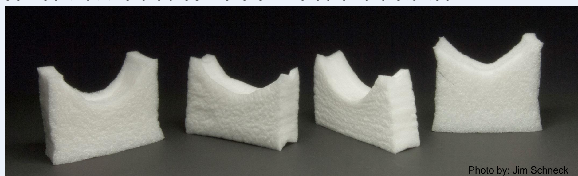
Cradles – shriveled and distorted 24 hours after being removed from a CO 2 treatment Photo by: Jim Schneck
